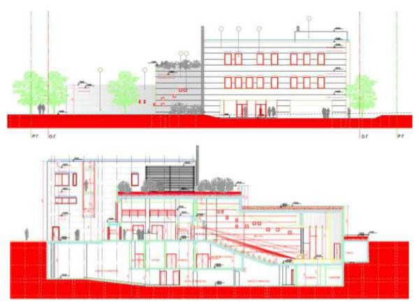
Architectural Elevation and Cross Section of the Building
